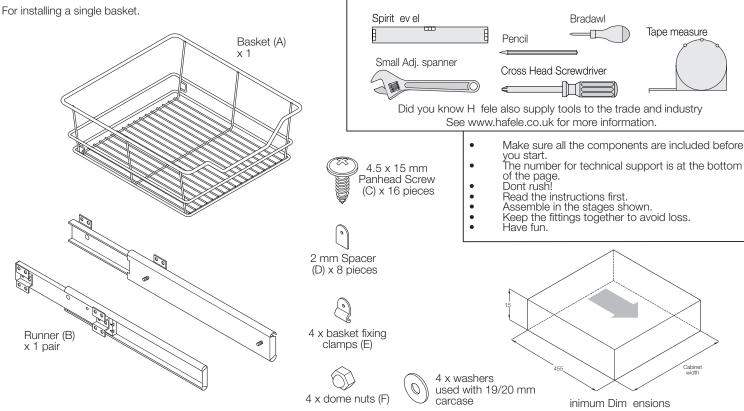
Using the runner drilling pattern shown in diagram 1, fix the runner (B) using 16 x 4.5 x 15 mm panhead screws (C) to the internal side of the carcase with the bottom runner fixing point a minimum of 55 mm up from the floor level of the cabinet. Then add the required no. of spacers for the carcase thickness being used to the threads on each runner.
