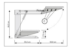
**4.4.2** Fix the upper part of the Kitchen appliance lift to the wall **(B)**. Fill the space between the Kitchen appliance lift and the wall with a suitable wooden joist. From above
