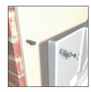
Secure the unit to brick and concrete block substrates using four 10 gauge x min.75 mm wood screws into proprietary wall plugs. The flat fender washer is to be inserted underneath the finishing washer. Finally, insert the snap-fit plastic covers in each fixing port to cover the fixings.
