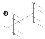
9 Fix 3 door plates (The door plate with the central hole is used later) to the door panel using 4 x M4 x 15 mm self tapping screws for each plate.
