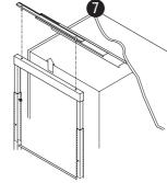
8 If a false double door effect is to be used, then connect the two door panels using the 2 door panel connectors and 8 x M4 x 15.0 mm pan head screws.
