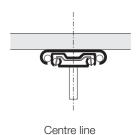
2 Repeat the same procedure in the top of the cabinet by finding and drawing the centre line. Position the top runner 5 mm from the front edge of the cabinet then align with the centre line on the top panel, pre drill 2 x 5 mm x 12 mm deep holes 40 mm and 265 mm from the front of the cabinet. Reposition the top runner 5 mm from the front edge of the cabinet and secure using 2 x Euro screws and 2 x M4 x 15.0 mm pan head screws using 2 adjacent holes located at the back of the slide.
