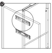
Finally insert the basket pins through the desired holes in the frame then secure using the pin caps. The baskets should be fit so that the bottom bar of the basket rests on the basket pins.
