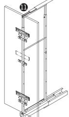
Hook the door onto the frame strips and tighten the screws to secure the frame strips to the door plates. Loosely fit 2 more M5 x 10 mm screws into the remaining holes inn the frame strips, these can be used for adjustment.
