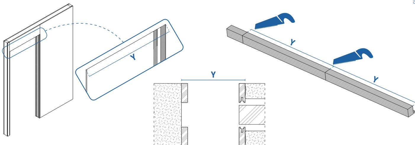
For 35 mm Doors - Cut brushes (D) to dimension  $Y$  and insert into both headers (C)
