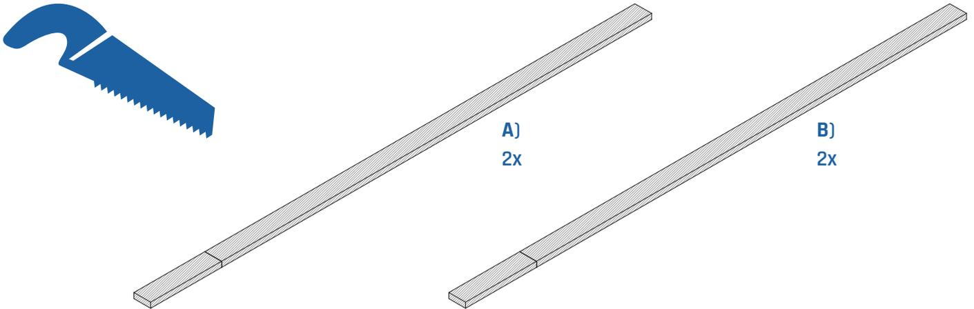
If the framework is not installed at finished floor level then cut A and B as shown below
