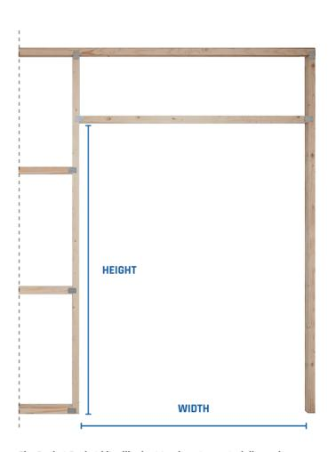
The Rocket Pocket kit will adapt to almost any stud dimension HOWEVER, the stud immediately above the frame must be 90 mm. You can add layers of plasterboard to this to then obtain the wall thickness you require. Bare in mind the jamb dimensions will change accordingly.
