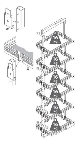
IMPORTANT - The unit has a maximum loading limit of 100kg. Load should be evenly distributed across all trays with maximum load capacity for each tray not exceeding 16kg.
