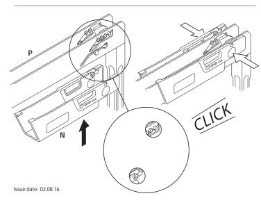
4 Insert the top into the bottom frame, and then attach this assembly to the bottom runner.
