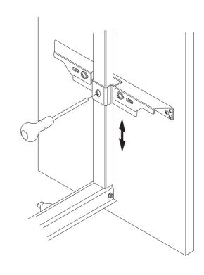
11 Adjust the vertical alignment of the door with the Alen screw located under the bottom runner.
