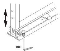
'Fine' adjustment of the vertical alignment of the door can be achieved by compressing the stop cover and sliding towards the front or rear.
