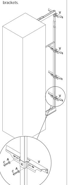
**8** Attach the tray mounting clips to the frame and insert the trays.
