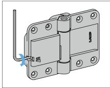
The door closing speed can be adjusted with a hex key (nominal 2.5).
