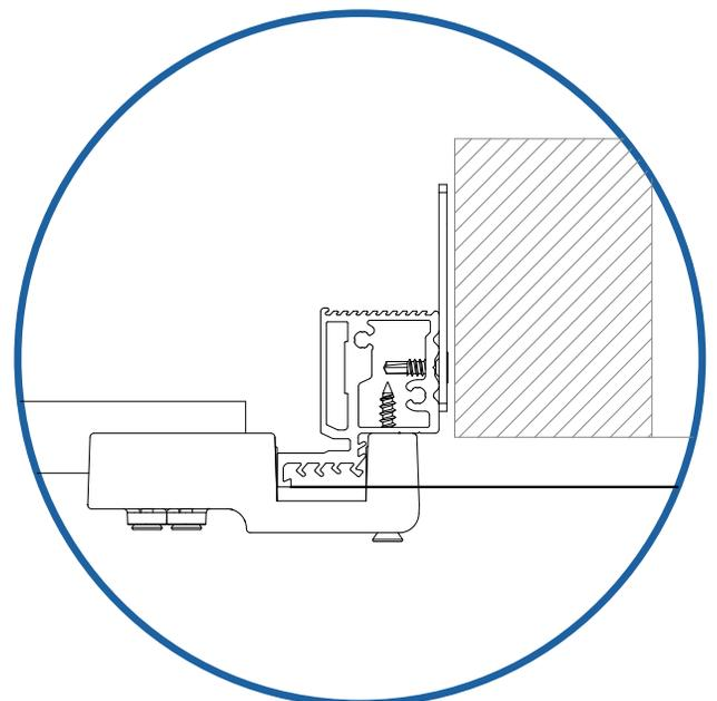
Make sure the frame is level and plumb and fix it to the studwork using brackets (i)
