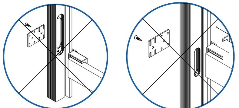
Place the frame into the studwork based on the chosen opening (push or pull).
