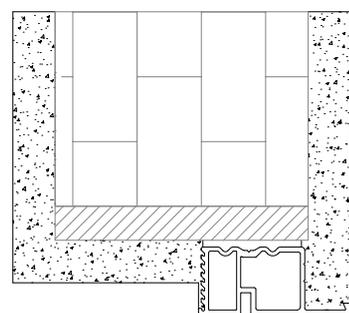
Apply fiberglass tape inbetween the frame and plasteboard, before plastering.
