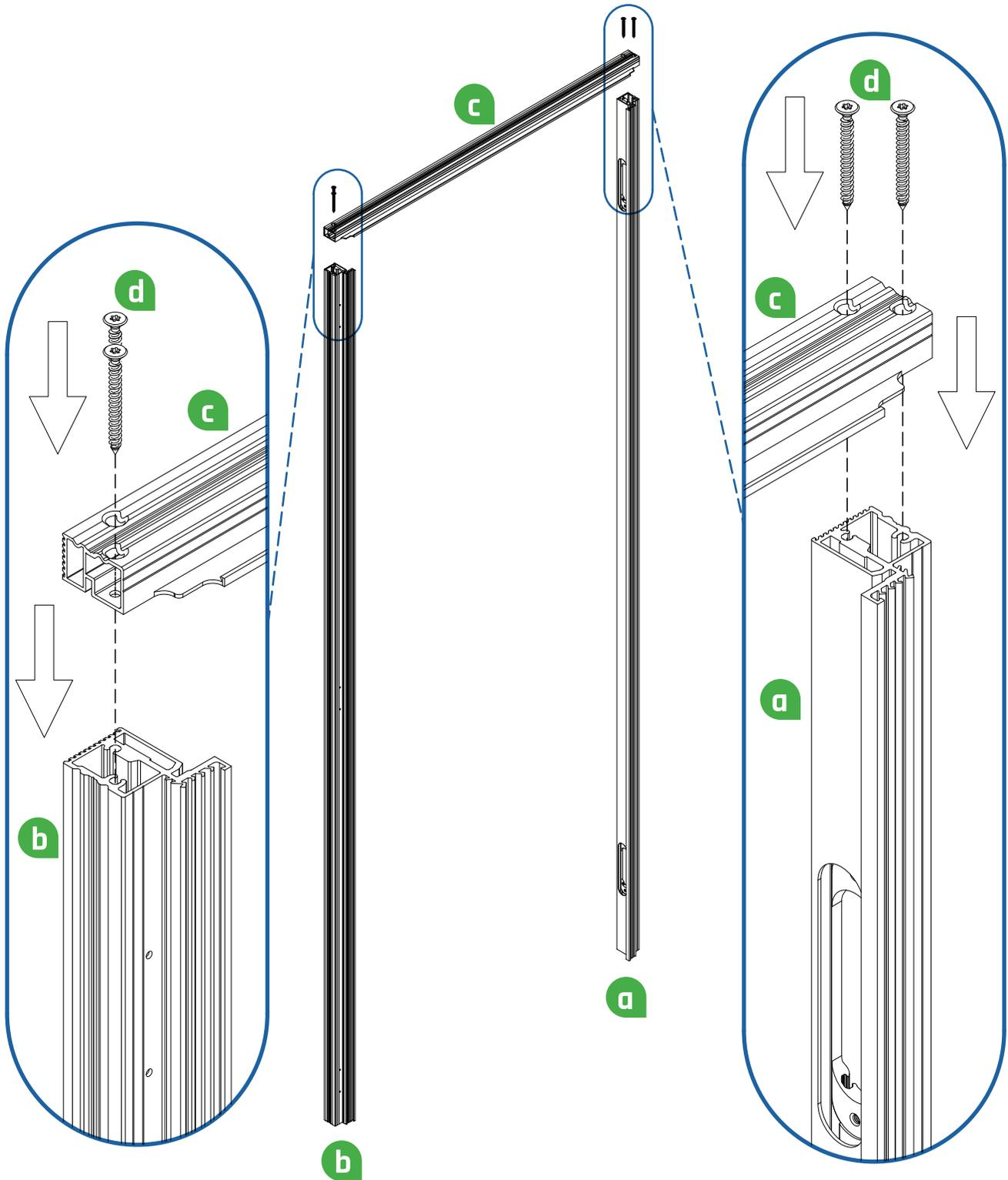
Join the two verticals (a+b) with the horizontal (c), taking note of where the hinge cut out are positioned like shown below. Use the supplied screw bit (m) to fix the screws (d) into the top of (c)
