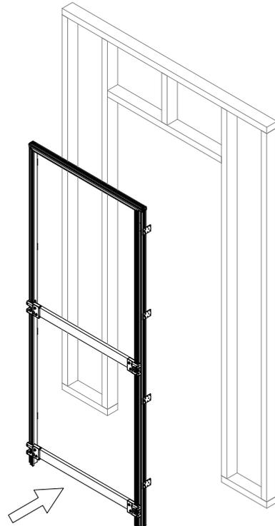
**ATTENTION:** make sure the frame is installed flush with the FINISHED wall level (including plasterboard)
