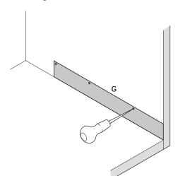
2 Secure runners to cabinet using 5 screws each side. On door hinge side, also use spacer provided, using longer fixing screws **A**.
