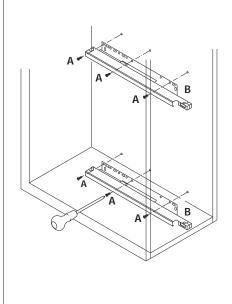
3 Slide carriage onto runners ensuring the carriage sits under the back retaining lugs, and click into place.
