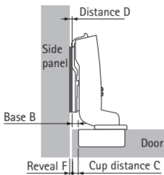
$$\begin{aligned} \text{Distance D} &= C + B + F \\ &= \text{cup distance C} - 4 \text{ mm} + \text{reveal F} \end{aligned}$$
