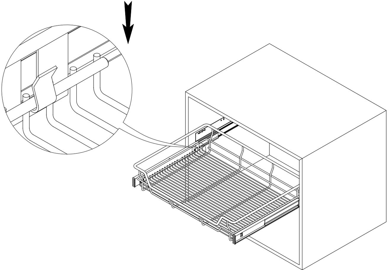
The four screws on the runner provide horizontal adjustment if necessary.
