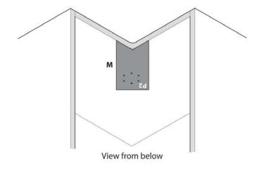
6 Insert carousel frame into base unit and align top and bottom mounting discs with pilot holes. When the runners are extended, there should be an equal distance on both sides between the runner and the cabinet side.
