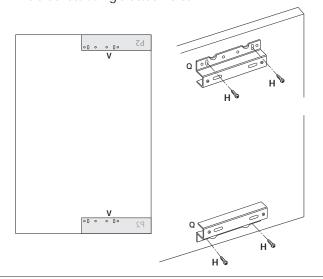
6 Insert 'L' shaped upper and lower door arms into side runner carriage frame tubes and secure lower door arm with two screws ensuring upper screw locates threaded hole in arm.
