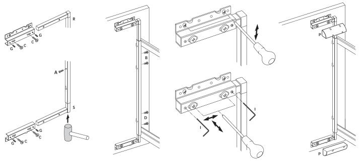
7 Fit door stop to restrict door mechanism opening
