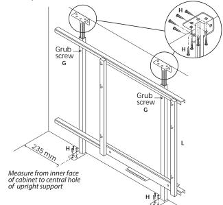
Place side runner carriage frame against cabinet side and align top and bottom to cabinet front edge.
