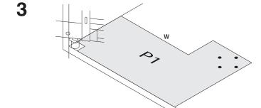
Place paper template (P1) on cabinet base and mark hole positions for swivel plate.
