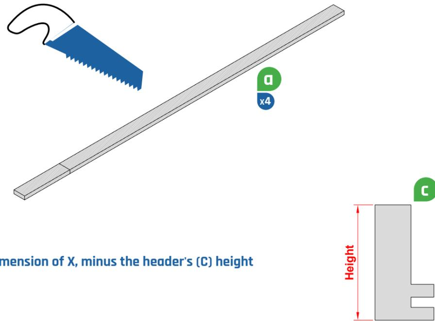
Cut verticals (A) to the dimension of X, minus the header's (C) height
