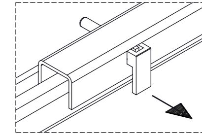
Unlock the slides and remove the wire structure
