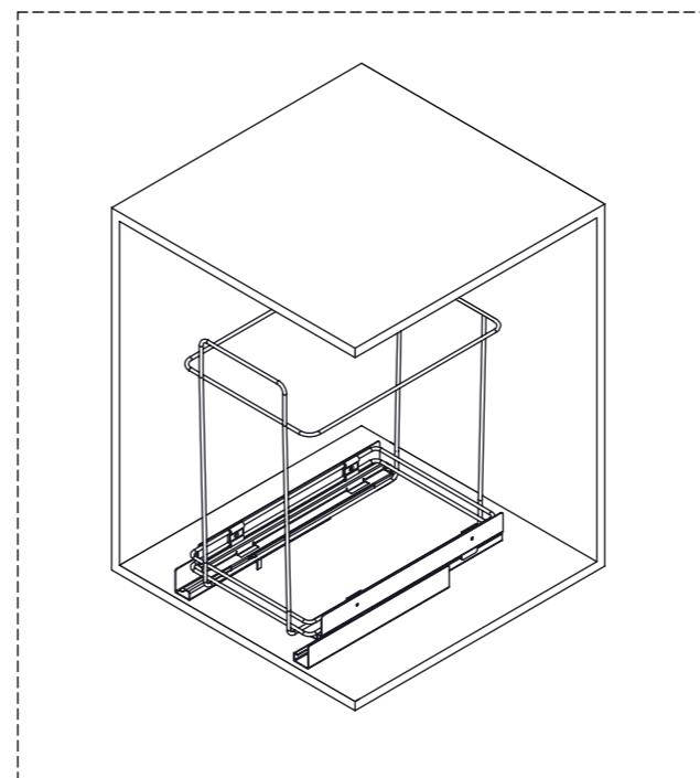
Place the wire structure back on the slides
