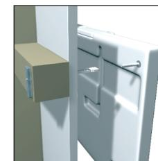
**5** Align and engage the fixing bolt in the threaded toggle bar with washers engaged. The flat fender washer is to be inserted underneath the finishing washer. Finally, insert the snap-fit plastic covers in each fixing port.
