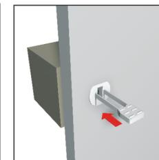
**4** Cut off the surplus projection of the toggle and offer up the unit for fixing.
