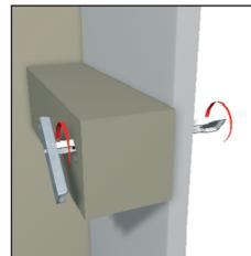
**3** Push the integral disc along the toggle to make a snug purchase on the wall face. The toggle strands are ratcheted to hold the disc in place.
