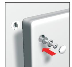
• In all mountings, the flat fender washer must be inserted underneath the finishing washer: installing the unit using only the finishing washer may result in the washer biting directly into the polyethylene body with consequent damage and loss of stability.
