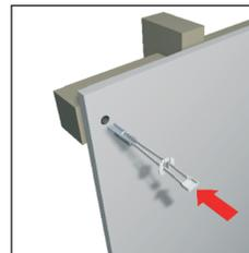
**2** Twist toggle freely to gain purchase on the supporting member. There should be a minimum cavity clearance of 65mm to allow the toggle bar to turn.
