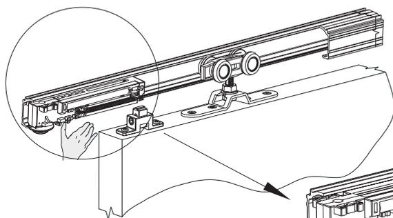
The soft close trigger needs to be activated before the first operation
