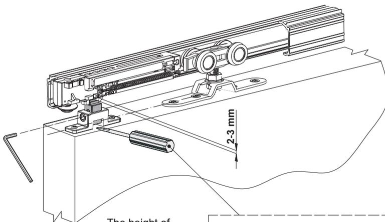
The height of the soft close catch needs to be adjusted once the door is fitted
