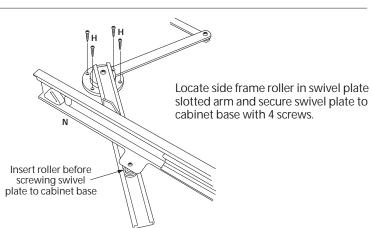
4 Attach linkage to rear runner carriage.
