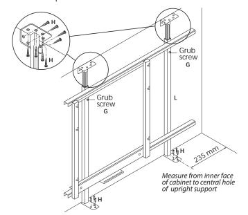
Place side runner carriage frame against cabinet side and align top and bottom to cabinet front edge.
