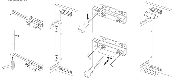
7 Fit door stop to restrict door mechanism opening
